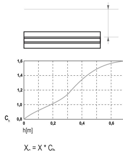
Adjusted range = range x  $C_h$ , where  $h$  on the chart is the distance from the ceiling to the grate.
